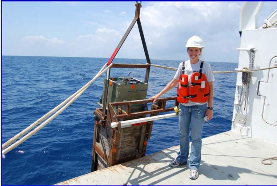
Figure 8. Laura Lapham holding on to the ROV docking bar of the Pore Fluid Array. The green box contains four osmo-samplers and rests on the 2000 pound drive weight.
