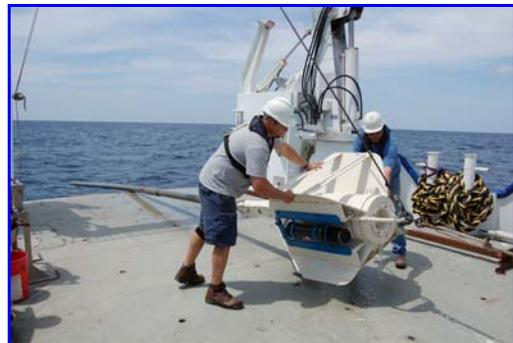
Figure 3. 10m core barrel on deck with USBL transponder connected to top of corer.
