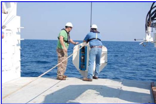
Figure 2. USBL transponder (dark gray pressure vessel in blue mount) connected to the weight of the gravity corer.
