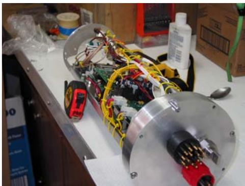
Figure 3. The communications and control computer system prior to encasement in the pressure vessel.
