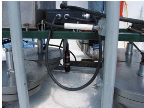
Figure 4. Lower side of the DeepSee with camera, altimeter, adjustable ballast system and pressure-compensated junction box within the field of view.
