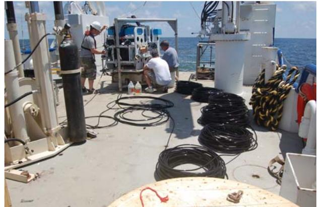
Figure 7. Array cable coiled on the deck of the *Pelican*.
