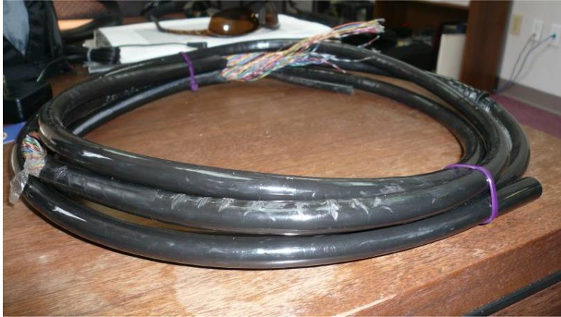
Figure 8. A damaged section of the resistivity array cable with bite marks, damaged jacket, and frayed wires.
