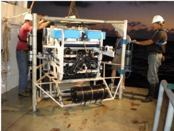
Figure 6. The electronics' package for the Resistivity Survey mounted to the front of the SSD lander cage.
