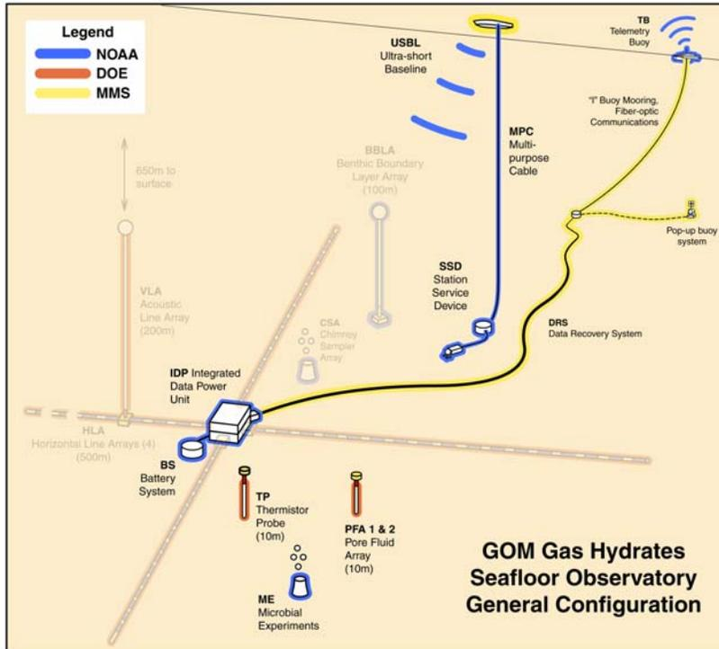
Figure 3. Cartoon of current configuration of the observatory. The IDP, DRS and Pop-up Buoy were deployed during this cruise. Color coded legend indicates contributions by major sponsors.
