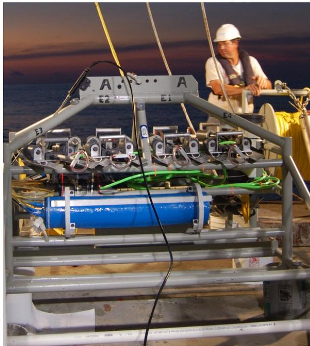
Figure 2. The Integrated Data/Power unit on the deck of the *Pelican* prior to deployment. The ROV latch-on bar is in the foreground and the central electronics package (blue) is mounted below a bank of underwater, ROV make-and-break connectors.
