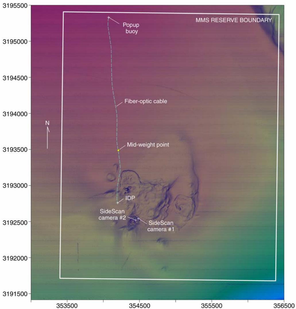
Figure 5. Site map of MC118 reserve area with locations of the IDP, DRS and Cameras deployed on this cruise.
