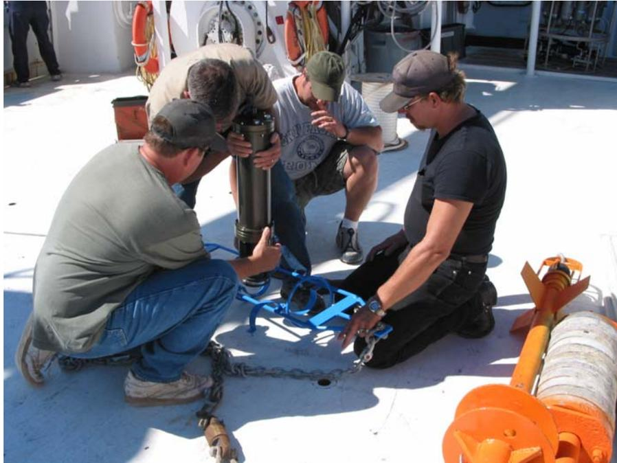
**Figure 3. CMRET and SDI technical teams mount the transponder in its protective “cage.”**
