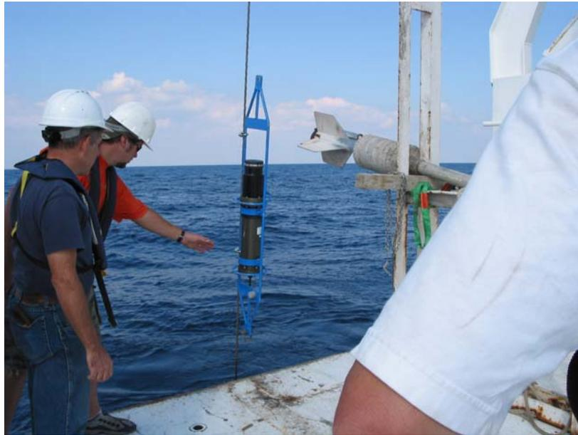
**Figure 4. USBL transponder attached to the cable supporting the gravity corer.**
