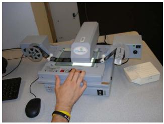
Push the tray back until the film is under the lighted area. Use the gray and red buttons to forward the film.
