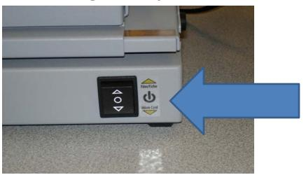
Switch to "Micro Card" mode on the front of the scanner.
