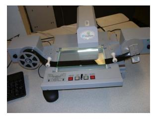
Pull out the gray tray until the glass pops up. Load the film, following the directions on the diagram on the tray.
