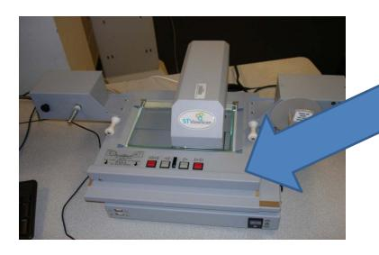
Pull out tray until glass pops up. Slide card under glass. Push the tray back until image is under the light. Start the ST ViewScan program. Use Browse tab to align and scan full pages.
